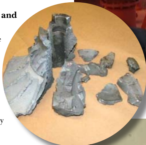
Fragments of a damaged turbo charger
